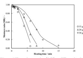
Figure 4 The moisture ratios (MR) at different heating times of the resulting MSW pellets (the initial moisture content was 50 wt.%) with the quantities of 15-30 g heated at the microwave power of 600 W.
