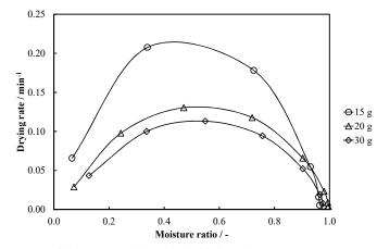
**Figure 6** The drying rate curves of the MSW pellets (the initial moisture content was 50 wt.%) with the quantities of 15-30 g heated at the microwave power of 600 W.
