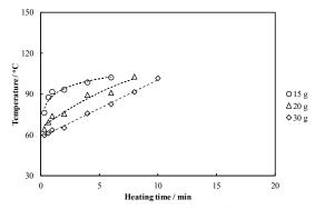
**Figure 5** The temperatures at different heating times of the resulting MSW pellets (the initial moisture content was 50 wt.%) with the quantities of 15-30 g heated at the microwave power of 600 W.
