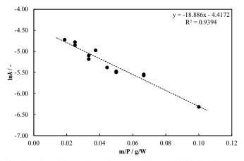
**Figure 7** The modified Arrhenius plot of the drying of MSW pellets (the initial moisture content was 50 wt.%) with the quantities of 15-30 g heated at the microwave powers of 300-800 W
