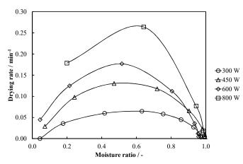
**Figure 3** The drying rate curves of the MSW pellets (the initial moisture content was 50 wt.%) with the quantity of 20 g heated at the microwave powers of 300-800 W.
