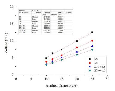
Figure 3 The graph of the relativity between applied electric current ( $\mu$ A) and the voltage (mV)
