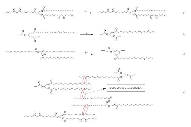
Figure 1 Radical initiation by UV radiation of a) ESO, b) tung oil, and c) linseed oil. d) the propose model of crosslinking among tung oil, linseed oil, and ESO
