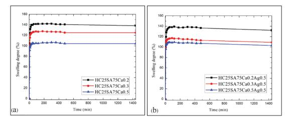
**Figure 2** Degree of swelling of HC/SA hydrogel films in distilled water at 37 °C. (a) HC25SA75 with varying concentrations of CaCl<sub>2</sub> as crosslinking agent; (b) HC25SA75 with varying concentrations of CaCl<sub>2</sub> and containing AgNPs.
