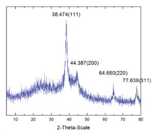
Figure 1 The XRD pattern of HC25SA75Ca0.5Ag5
