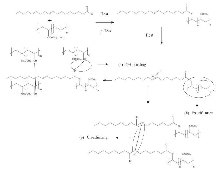
Fig.1. The proposed reactions of PVA and Oleic acid
