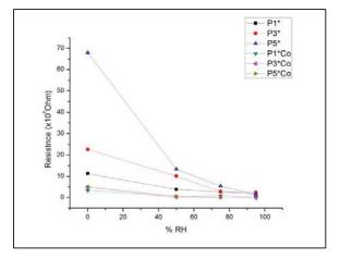
Fig.4. Humidity sensing properties of P\* films
