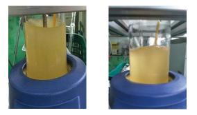
(a) Stirrer mixing (b) Nitrogen microbubble mixing
