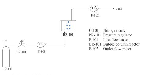
Figure 3 Biodiesel production by microbubble mixing system
