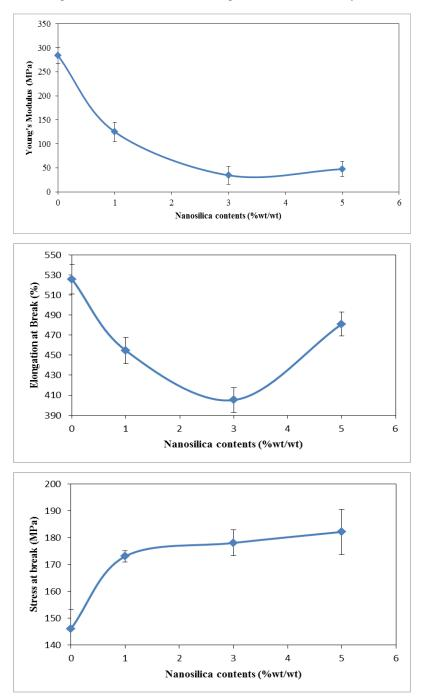
Figure 3 Mechanical properties of nylon /nanosilica fibers versus nanosilica content of: (a) Young's modulus (b) elongation at break and (c) stress at break.
