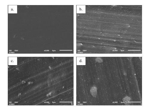
**Figure 2** SEM cross section images of (a) neat nylon and composites of (b) 1% nanosilica, (c) 3% nanosilica and (d) 5% nanosilica in nylon fibers.
