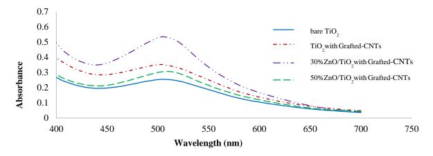
Figure 5 UV-vis absorption spectra of photoanodes.
