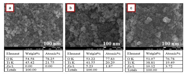
**Figure 3** FE-SEM images (scale bar: 100 nm) with EDX analysis of (a) bare  $TiO_2$ , (b) 30% ZnO/TiO<sub>2</sub> and (c) 50% ZnO/TiO<sub>2</sub>
