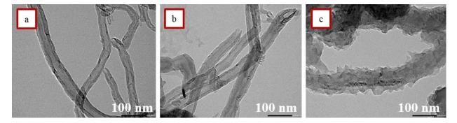
**Figure 2** TEM images (scale bar: 100 nm) of (a) bare CNTs and gratefed-CNTs with poly(vinyl acetated):polyaniline at (b) 0.4:1 and (c) 1:1 ratios
