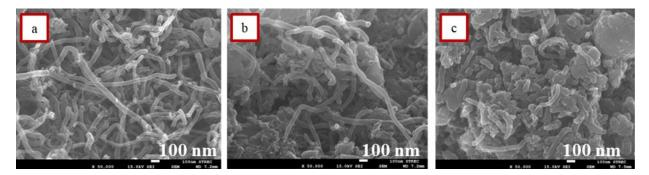
**Figure 1** FE-SEM images (scale bar: 100 nm) of (a) bare CNTs and gratefed-CNTs with poly(vinyl acetated):polyaniline at (b) 0.4:1 and (c) 1:1 ratios
