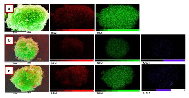
Figure 4 Mapping images of (a) bare TiO<sub>2</sub>, (b) 30%ZnO/TiO<sub>2</sub> and (c) 50%ZnO/TiO<sub>2</sub>
