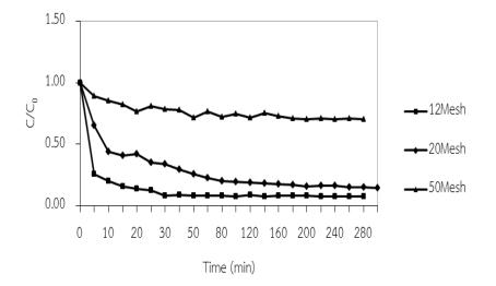
Figure 4 Removal of MB dye at various mesh sizes for the adsorbent derived from CBP
