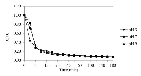
Figure 7 Removal of MB dye at various pH values for the adsorbent derived from CBP
