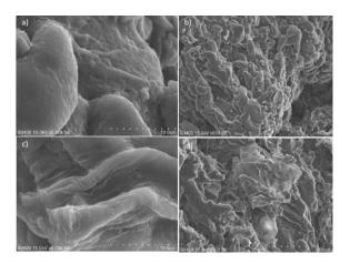
**Figure 3** SEM micrographs of (a) CBP (magnification: 5.00 K), (b) CBP (magnification: 500), (c) SBBP (magnification: 5.00 K), (d) SBBP (magnification: 500)
