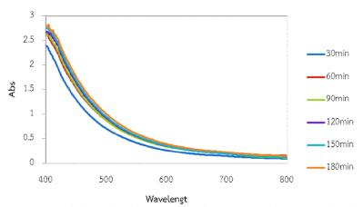
Figure 2 The absorbance spectra of adsorption via banana sap in water at various adsorption times.
