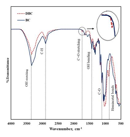
Figure 3 FT-IR spectra of BC and DBC
