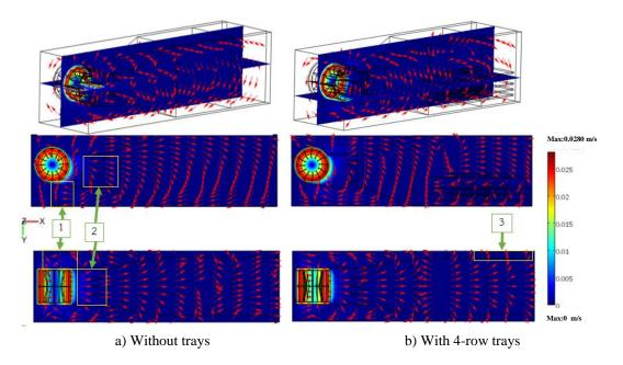
Figure 2 Hot air circulation i.e. velocity vectors and contours
