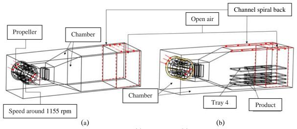
**Figure 1** Geometry of oven and control boundaries (a) without trays (b) with 4-row trays; velocity arrows indicating flow circulation.
