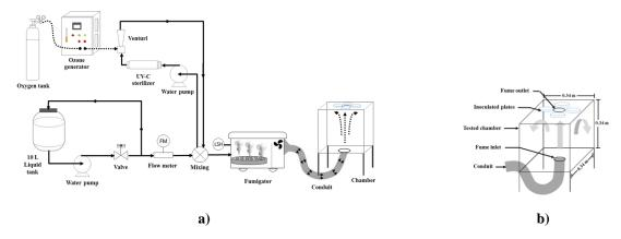
**Figure 1** a) The schematic diagram of AOPs aerosolization and b) Diagram of the testing chamber made of transparent walls. Disinfectant fume is introduced from the bottom and exited at the outlet on top.
