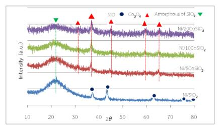
Figure 1 The XRD pattern of the Ni/CoSiO<sub>2</sub> catalyst with various Co loadings
