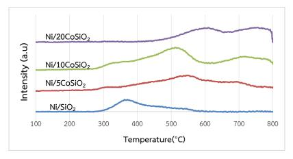
Figure 2 TPR profiles of the Ni/CoSiO<sub>2</sub> catalyst with various Co loadings
