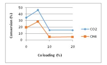
Figure 3 CH<sub>4</sub> and CO<sub>2</sub> conversions for the DRM on the Ni/CoSiO<sub>2</sub> catalyst with various Co loadings
