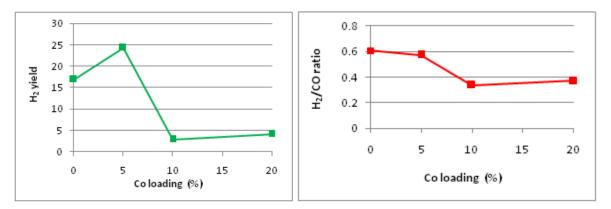
Figure 4 H<sub>2</sub> yield and H<sub>2</sub>/CO ratio in the product for the DRM on the Ni/CoSiO<sub>2</sub> catalyst with various Co loadings
