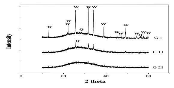
**Figure 2.** XRD patterns of glazes G1, G11 and G21 heat-treated at 1250 °C and soaking time at 1100 °C for 4 hour; Q = Quartz and W = Willemite
