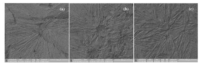
**Figure 3.** Microstructural analysis of glazes heat-treated at 1250 °C and soaking time at 1100 °C for 4 h ; (a) G1, (b) G11 and (c) G21
