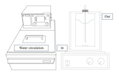
Figure 2 The set-up of solubility measurements
