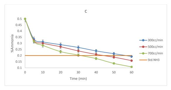
**Figure 2** The remaining  $NH_3$  content (wt%) after flowing of air for 60 minute through diffusers P2(a), P3(b), and P4(c) at air flow rates of 300, 500 and 700 cc/min.
