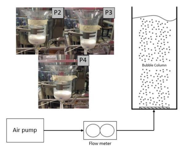
**Figure 1** Experimental setup for ammonia removal via bubbles .The inset is a photograph of the bubble column while flowing air with a flow rate 300 cc/min through a diffuser P2, P3, and P4.
