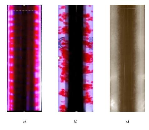
Figure 2: Comparison of two-phase Taylor-Couette flow for  $B = 14 \text{ m}^3\text{m}^2\text{h}^{-1}$ ; a)  $D_i/D_C = 0.8$ , n = 950 rpm b)  $D_i/D_C = 0.5$ , n = 1000 rpm and c)  $D_i/D_C = 0.5$ , n = 1200 rpm; Continuous phase: water, dispersed phase: Shellsol-T; Temperature: ambient
