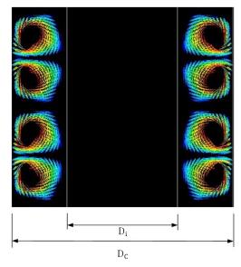
Figure 1: Flow pattern from CFD simulation of two-phase Taylor-Couette flow for  $D_i/D_c = 0.5$
