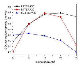
Figure 4 CO<sub>2</sub> adsorption capacity of 1:2TEPA30, 1:1TEPA30 and 1:0.5TEPA30 at different adsorption temperatures
