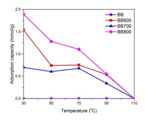
Figure 3 CO<sub>2</sub> adsorption capacity of BB with physical activation at different levels of adsorption temperature
