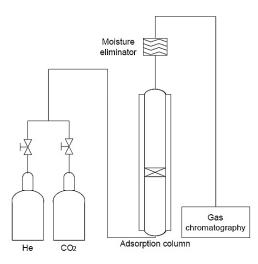
Figure 1 Experimental set-up for gas – solid adsorption column
