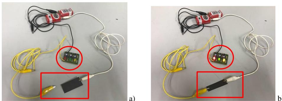
Figure 4 The simple circuit including LED (in circle) and the prepared conductive print (in square blanket) a) open circuit and b) closed circuit
