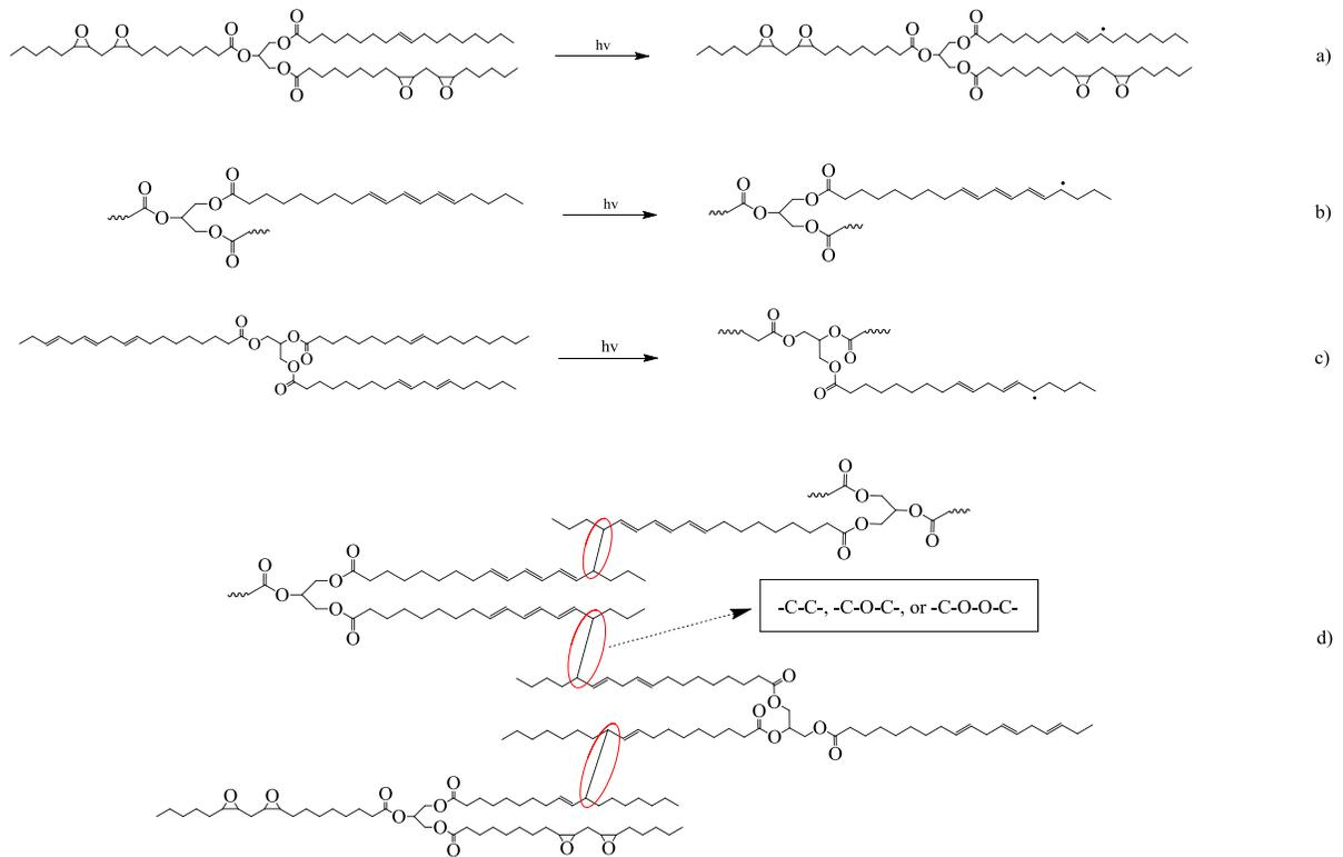
**Figure 1** Radical initiation by UV radiation of a) ESO, b) tung oil, and c) linseed oil. d) the propose model of crosslinking among tung oil, linseed oil, and ESO
