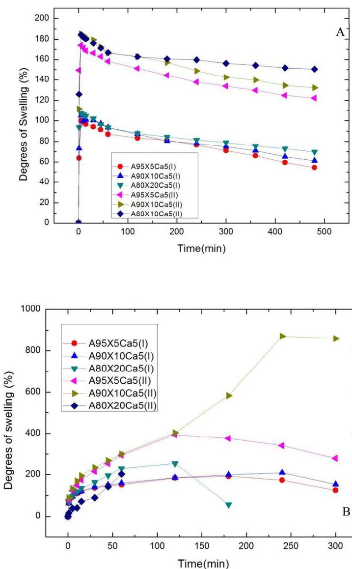
**Figure.2** Degree of swelling of A/X hydrogel films : (a) in SGF at 37 °C and (b) in SIF at 37 °C
