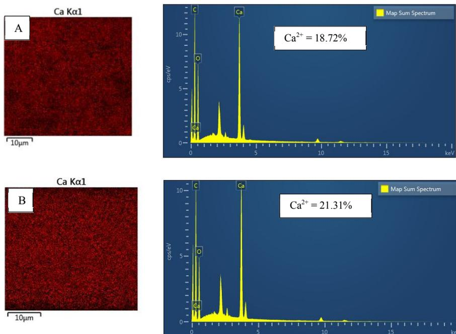
**Figure.1** Distribution of Ca<sup>2+</sup> ion on the cross-section of hydrogel films: (a) A95XCa5(I); (b) A95X5Ca5(II)
