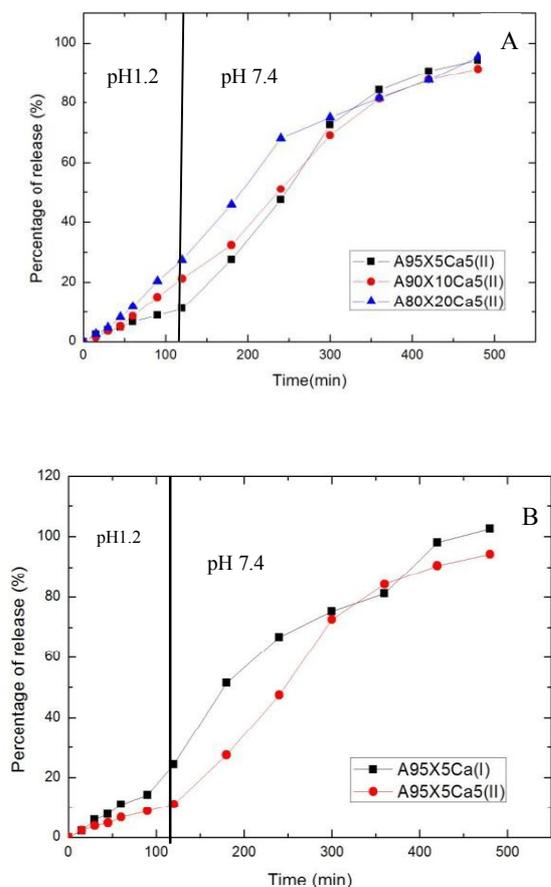
**Figure.3** The release profiles of paracetamol in SGF followed by SIF at 37 °C
