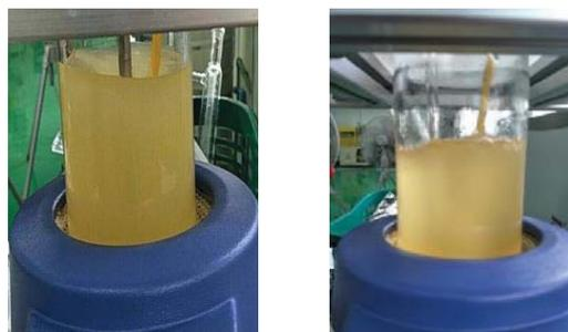
(a) Stirrer mixing (b) Nitrogen microbubble mixing
