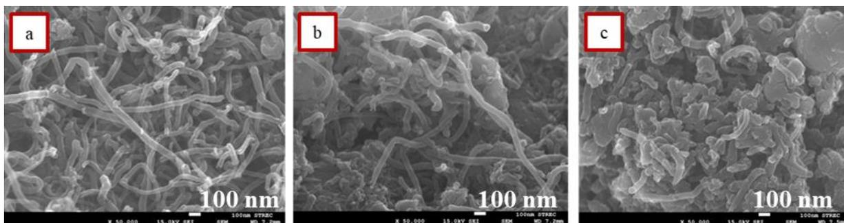
**Figure 1** FE-SEM images (scale bar: 100 nm) of (a) bare CNTs and grafted-CNTs with poly(vinyl acetate):polyaniline at (b) 0.4:1 and (c) 1:1 ratios
