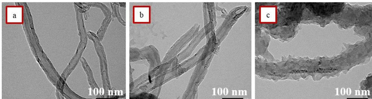
**Figure 2** TEM images (scale bar: 100 nm) of (a) bare CNTs and grafted-CNTs with poly(vinyl acetate):polyaniline at (b) 0.4:1 and (c) 1:1 ratios
