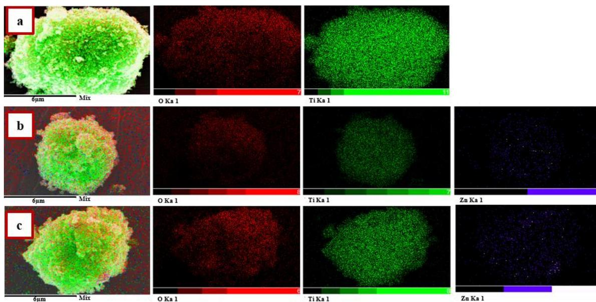
**Figure 4** Mapping images of (a) bare TiO<sub>2</sub>, (b) 30% ZnO/TiO<sub>2</sub> and (c) 50% ZnO/TiO<sub>2</sub>
