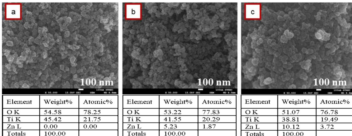
**Figure 3** FE-SEM images (scale bar: 100 nm) with EDX analysis of (a) bare TiO<sub>2</sub>, (b) 30% ZnO/TiO<sub>2</sub> and (c) 50% ZnO/TiO<sub>2</sub>
