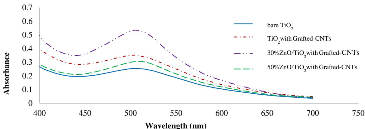
Figure 5 UV-vis absorption spectra of photoanodes.
