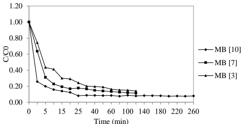
**Figure 6** Removal of MB dye at various initial concentrations of MB dye for the adsorbent derived from CBP
