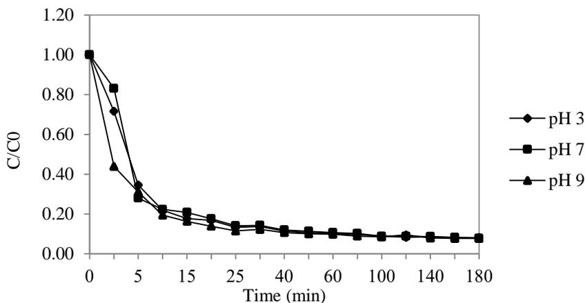
**Figure 7** Removal of MB dye at various pH values for the adsorbent derived from CBP
