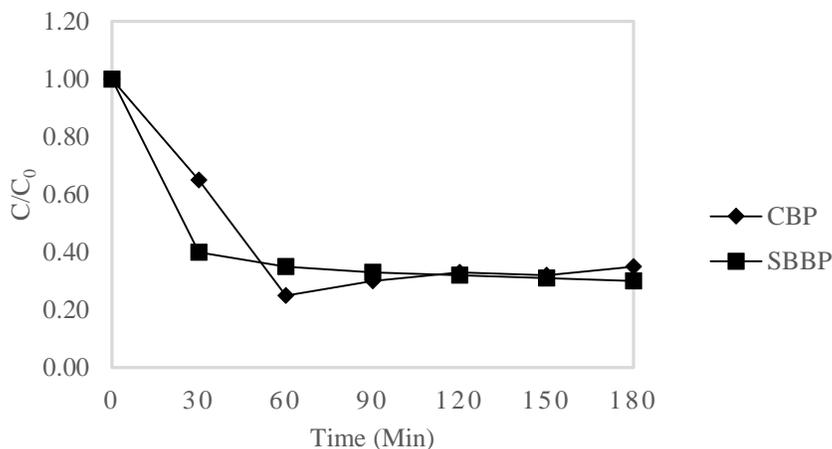
**Figure 1** Removal of MB dye from batch experiments by using CBP and SBBP at the condition: adsorbent size of 12 mesh, the initial MB dye concentration of 10 mg/L and adsorbent dosage of 20 g at 30 °C.
