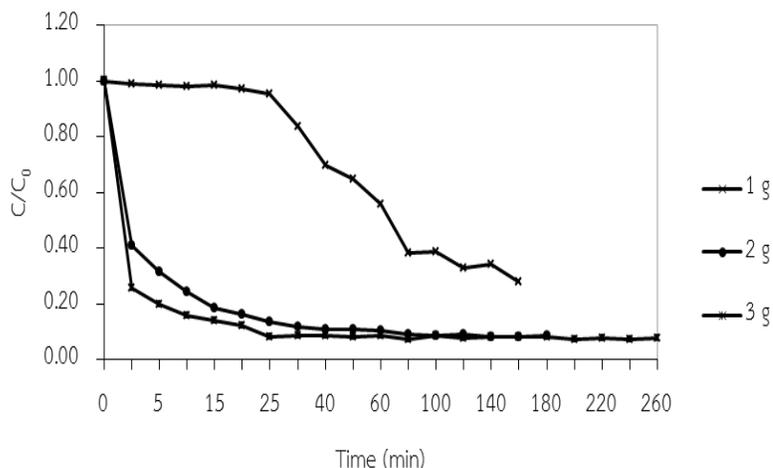
**Figure 5** Removal of MB dye at various adsorbent dosages for the adsorbent derived from CBP
