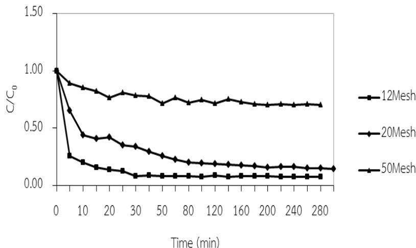
**Figure 4** Removal of MB dye at various mesh sizes for the adsorbent derived from CBP
