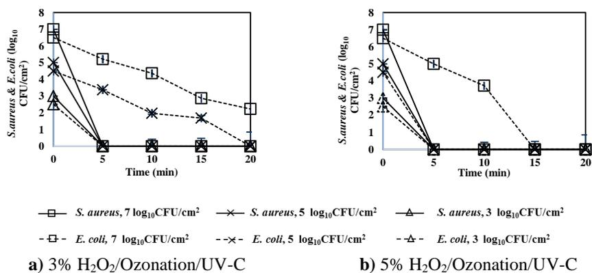
**Figure 3** Effect of H<sub>2</sub>O<sub>2</sub> concentrations combined with UV-C photocatalysis and ozonation. H<sub>2</sub>O<sub>2</sub> treatment on the initial cell 3, 5 and 7 log<sub>10</sub> CFU/cm<sup>2</sup> of *E. coli* and *S. aureus*
