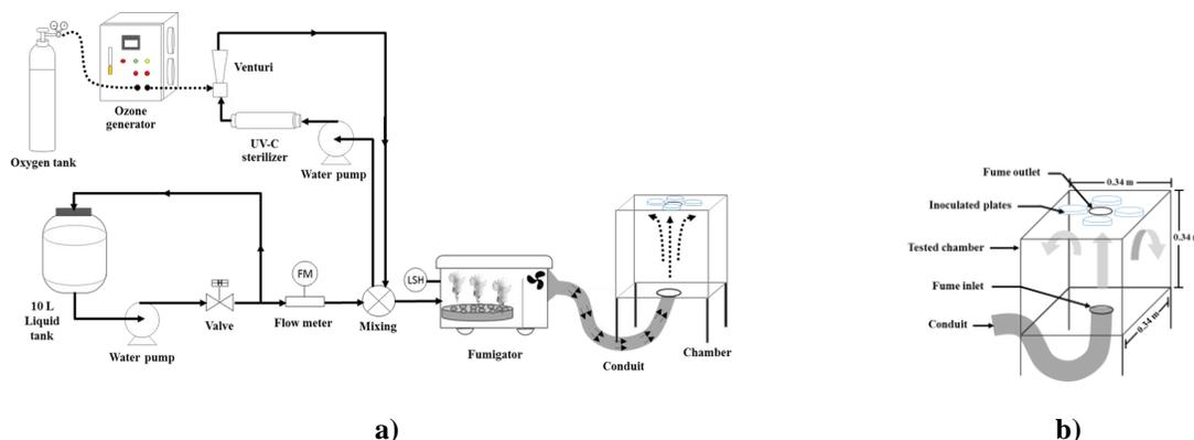
**Figure 1** a) The schematic diagram of AOPs aerosolization and b) Diagram of the testing chamber made of transparent walls. Disinfectant fume is introduced from the bottom and exited at the outlet on top.
