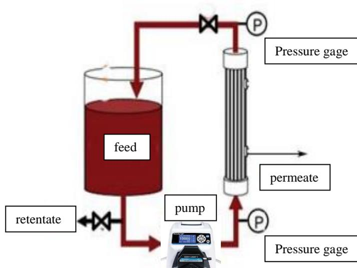
**Figure 1** The experimental set up for membrane separation (adopted from Kitsuwat et al. 2015)
