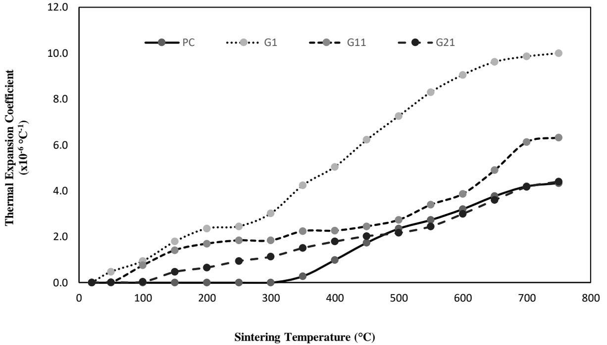
**Figure 1.** Plot of coefficient of thermal expansion; PC = porcelain clay, G1 = glazes formula 1, G11 = glazes formula 11 and G21 = glazes formula 21
