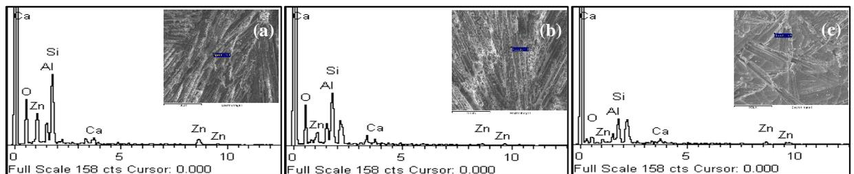
**Figure 4.** EDS analysis of glazes heat-treated at 1250 °C and soaking time at 1100 °C for 4 h ; (a) G1, (b) G11 and (c) G21
