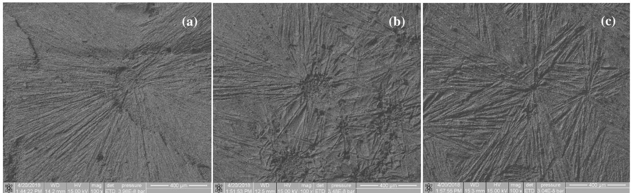
**Figure 3.** Microstructural analysis of glazes heat-treated at 1250 °C and soaking time at 1100 °C for 4 h ; (a) G1, (b) G11 and (c) G21
