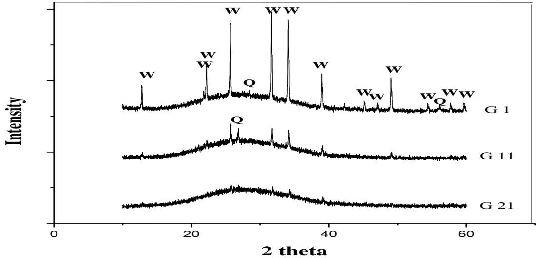
**Figure 2.** XRD patterns of glazes G1, G11 and G21 heat-treated at 1250 °C and soaking time at 1100 °C for 4 hour; Q = Quartz and W = Willemite
