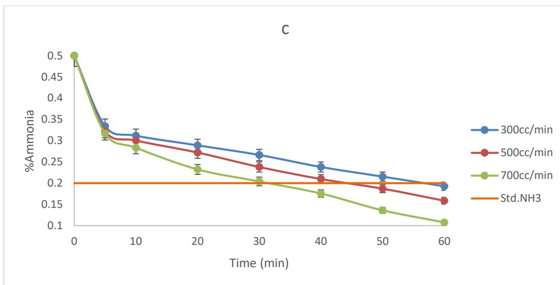
**Figure 2** The remaining NH<sub>3</sub> content (wt%) after flowing of air for 60 minute through diffusers P2(a), P3(b), and P4(c) at air flow rates of 300, 500 and 700 cc/min.
