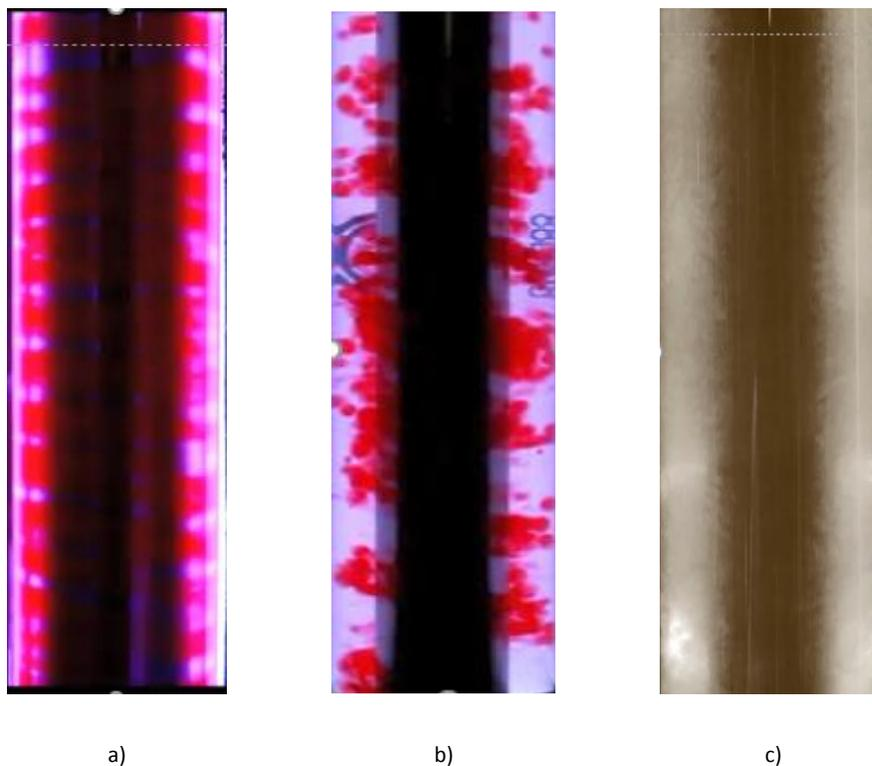
**Figure 2: Comparison of two-phase Taylor-Couette flow for  $B = 14 \text{ m}^3\text{m}^{-2}\text{h}^{-1}$ ; a)  $D_i/D_C = 0.8$ ,  $n = 950 \text{ rpm}$  b)  $D_i/D_C = 0.5$ ,  $n = 1000 \text{ rpm}$  and c)  $D_i/D_C = 0.5$ ,  $n = 1200 \text{ rpm}$ ; Continuous phase: water, dispersed phase: Shellsol-T; Temperature: ambient**
