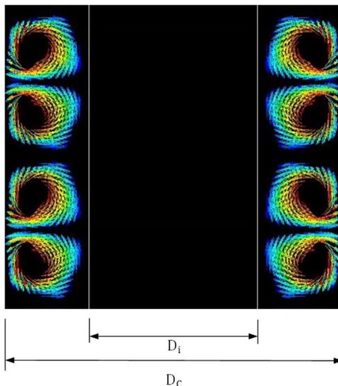
**Figure 1: Flow pattern from CFD simulation of two-phase Taylor-Couette flow for  $D_i/D_C = 0.5$**
